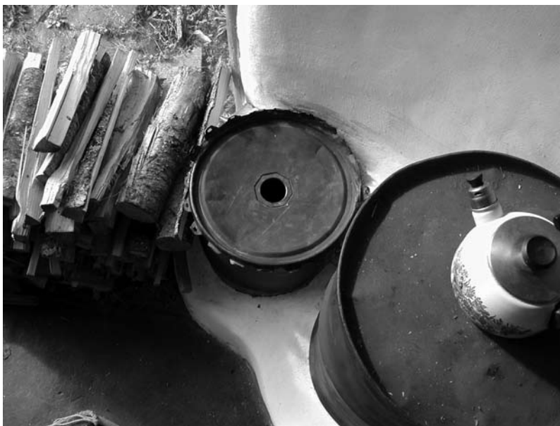
The Rocket Stove in Ianto Evans's cottage, seen from above. Dry firewood, cut thin, the small feed barrel with lid and the large heat riser barrel with tea kettle.
